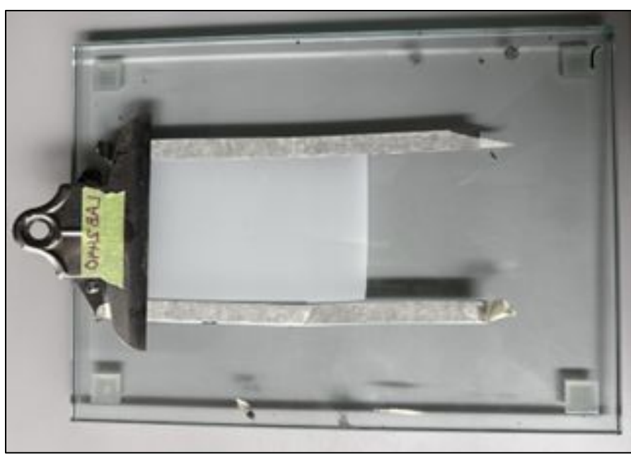
Figure 3. Foam Fabrication set up for Rolled 2mm samples.
